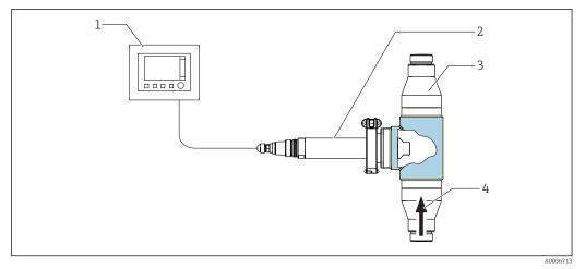
■ 1 Measuring system with CUA252 flow assembly
