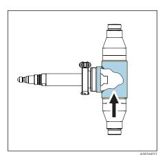
Installing with CUA252 flow assembly
