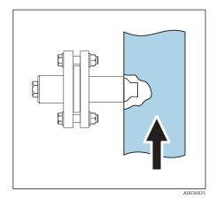
■ 12 Installing with CUA120 flow assembly
