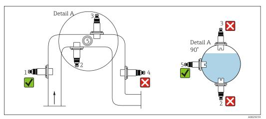
Permitted and unacceptable orientations in pipes
