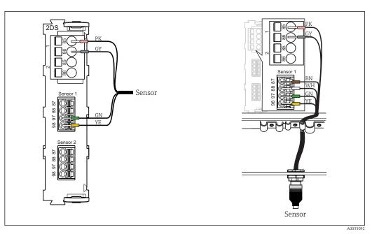
■ 5 Sensor connection to sensor input (left) or via M12 connector (right)
