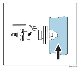
Installing with CUA451 retractable assembly
