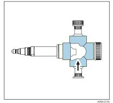
■ 15 Installing with CYA251 flow assembly
