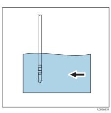
The installation angle is  $0^{\circ}$ .
