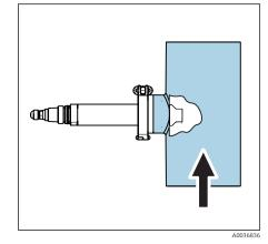
■ 14 Installing with CUA262 flow assembly
