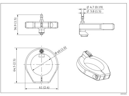
■ 20 Dimensions for compressed air cleaning. Dimensions: mm (in)
