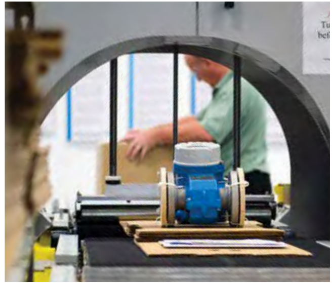
An electromagnetic flowmeter makes its way into the automatic shrink-wrap machine before it is boxed up and shipped to the customer
