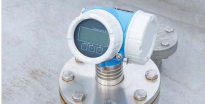
Guided wave radar
