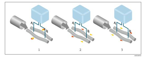
The phase difference (A-B) increases with increasing mass flow. Electrodynamic sensors register the tube oscillations at the inlet and outlet. System balance is ensured by the antiphase oscillation of the two measuring tubes. The measuring principle operates independently of temperature, pressure, viscosity, conductivity and flow profile.
