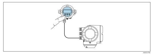
44 Operation via remote display and operating module DKX001
