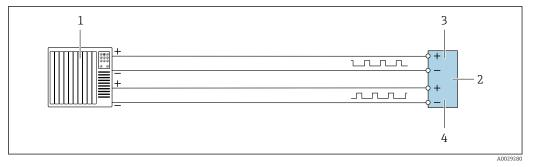
■ 16 Connection example for double pulse output (active)
