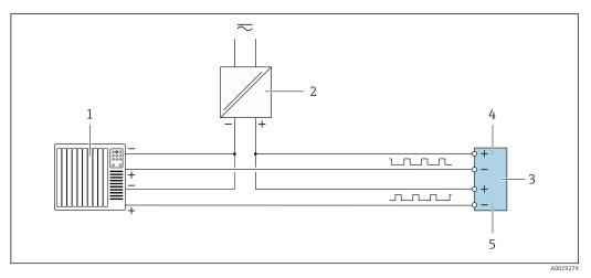
17 Connection example for double pulse output (passive)
