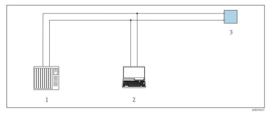
☑ 50 Options for remote operation via Modbus-RS485 protocol (active)
