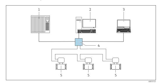
52 Options for remote operation via EtherNet/IP network: ring topology
