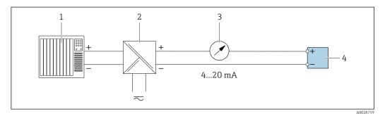
■ 13 Connection example for 4-20 mA current output (passive)
