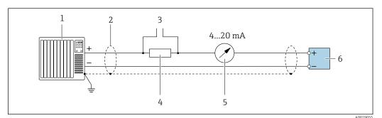
Connection example for 4 to 20 mA HART current output (active)
