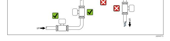
To prevent measuring errors arising from accumulation of gas bubbles in the measuring tube, avoid the following mounting locations in the pipe:
