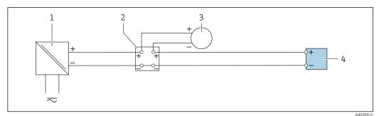
🖻 19 Connection example for 4 to 20 mA current input
