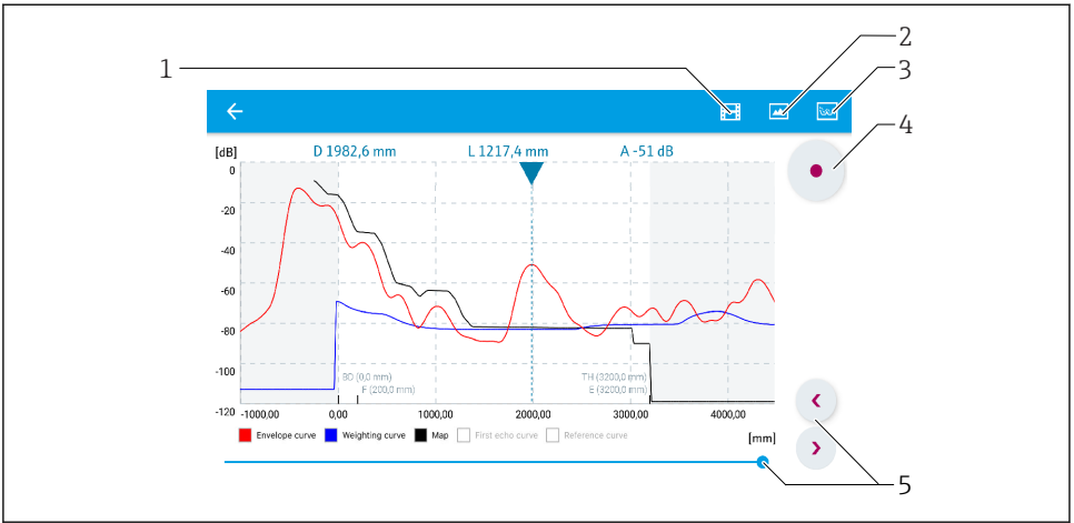
20 Envelope curve display (sample) in SmartBlue for Android
