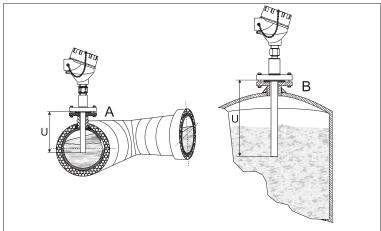
Examples of installation. In pipes of a small section the axis line of the duct must be reached and if possible slightly exceeded by the tip of the probe (=U).
