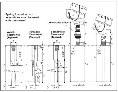
Note: \*For wells with ½" NPT - 1" Process thread length and ¾" Hex length dimensions are reversed.
