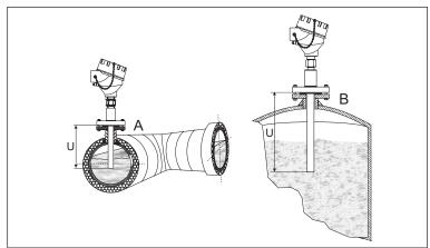
Examples of installation. In pipes of a small section the axis line of the duct must be reached and if possible slightly exceeded by the tip of the probe (=U).
