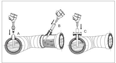
Examples of spring loaded insert installation.
