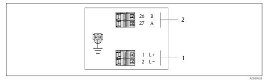
Modbus RS485 terminal assignment, connection version for use in non-hazardous areas and Zone 2/Div.
