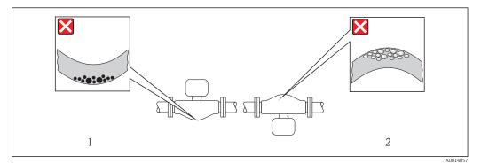
🖻 20 Orientation of sensor with curved measuring tube
