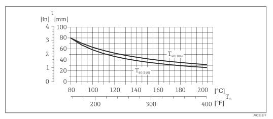
25 Maximum recommended insulation thickness depending on the temperature of the medium and the ambient temperature
