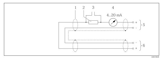
🖸 17 Connection example for HART input (burst mode) via current output (active)
