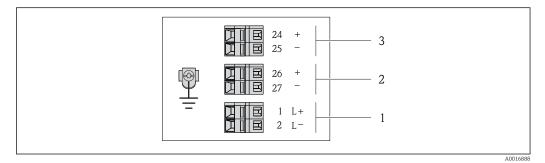
☑ 2 Terminal assignment 4-20 mA HART with pulse/frequency/switch output
