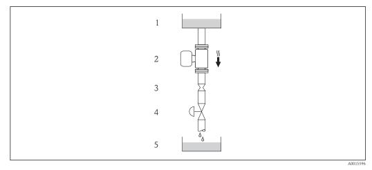
🛃 19 Installation in a down pipe (e.g. for batching applications)
