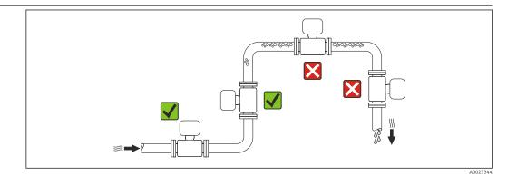
To prevent measuring errors arising from accumulation of gas bubbles in the measuring tube, avoid the following mounting locations in the pipe:
