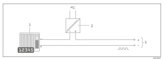
10 Connection example for pulse/frequency output (passive)
