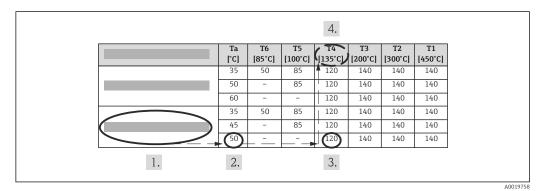
22 Procedure for determining the maximum surface temperature
