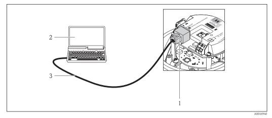
35 Connection for order code for "Output", option N: EtherNet/IP
