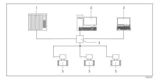
Options for remote operation via Ethernet-based fieldbus
