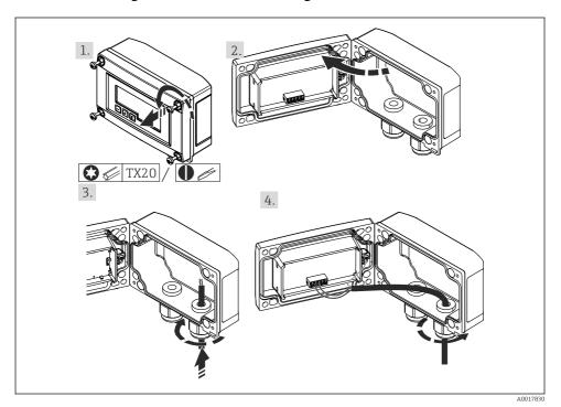
■ 8 Inserting the cable, field housing
