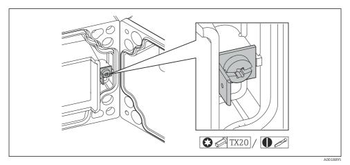
■ 10 Functional grounding terminal in field housing
