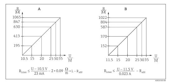
A FMX21 4 to 20 mA HART load chart for estimating the load resistance. Additional resistances, such as the resistance of the extension cable, have to be subtracted from the value calculated as shown in the equation.
