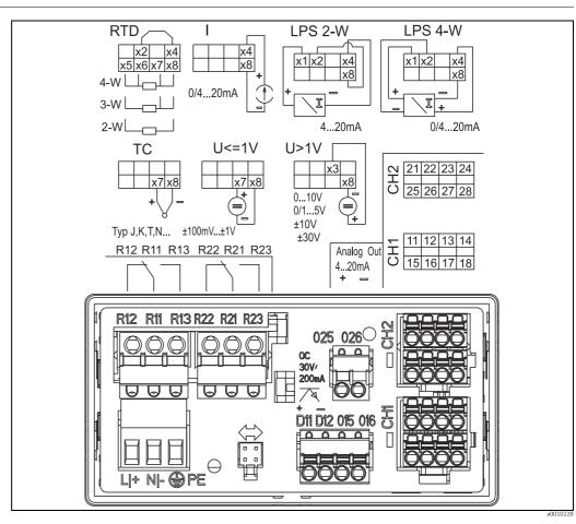
$Terminal\ assignment\ of\ panel\ meter\ (relays\ (terminals\ Rx1-Rx3)\ and\ channel\ 2\ (terminals\ 21-28\ and\ O25/O26)\ are\ optional)$
