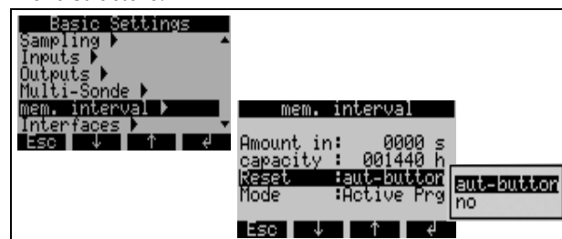
Fig. 17: Configuring the internal datalogger
