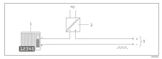
$\blacksquare$  7 Connection example for pulse/frequency output (passive)
