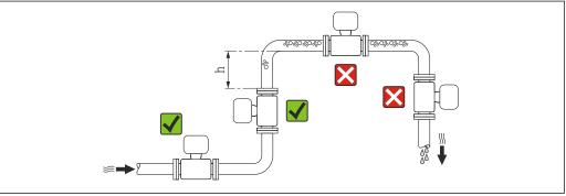
Preferably install the sensor in an ascending pipe, and ensure a sufficient distance to the next pipe elbow:  $h \ge 2 \times DN$
