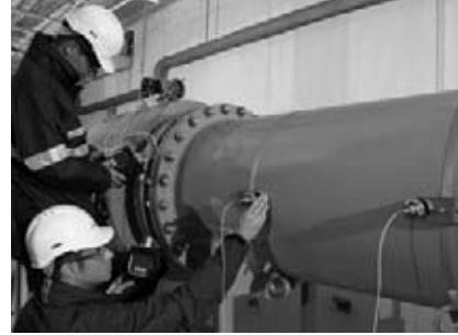
Prosonic Flow 93T used for the measurement consistency check of an electromagnetic flowmeter
