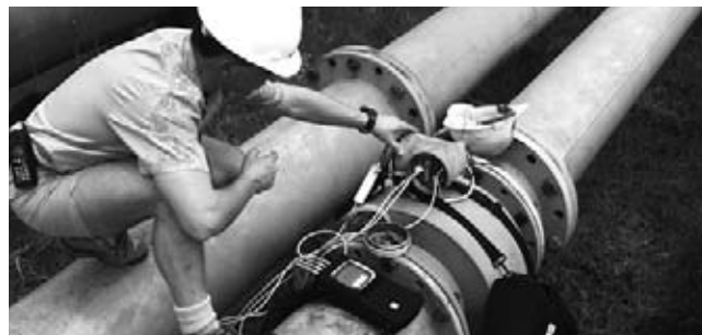
On-site functional check of a flowmeter using the FieldCheck.
