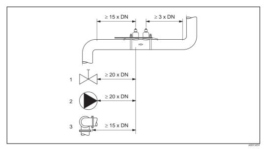
Fig. 5: Inlet and outlet run
