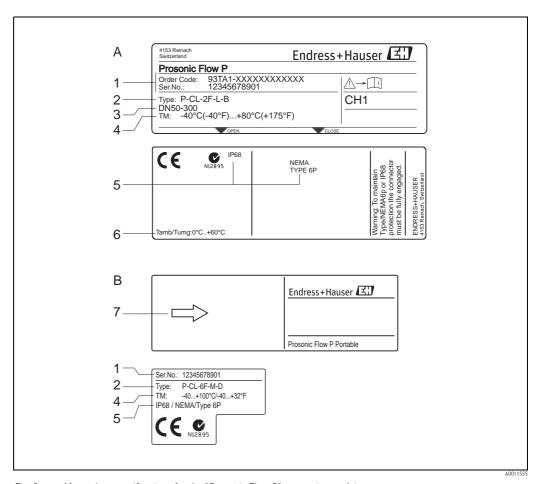
$\textit{Fig. 2:} \qquad \textit{Nameplate specifications for the "Prosonic Flow P" sensor (example)}$
