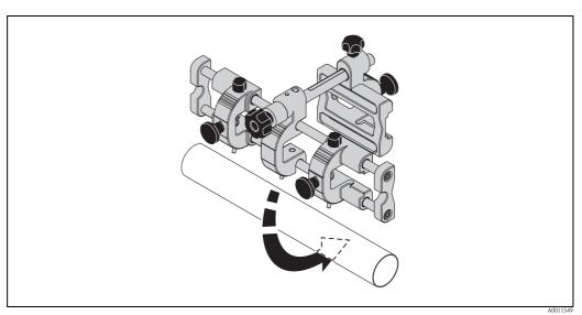
Fig. 9: Setting the sensor holder on the pipe
