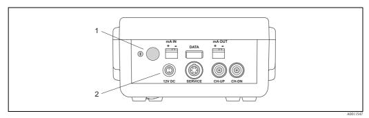
Fig. 7: Connecting and switching on the transmitter
