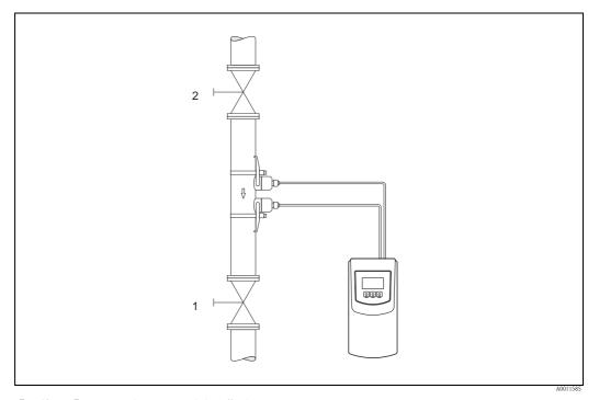
Fig. 43: Zero point adjustment and shutoff valves
