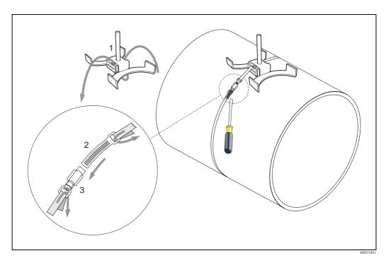
Fig. 17: Premounting strapping bands for pipe diameters DN > 200 (8")
