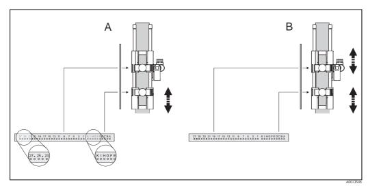
Fig. 12: Setting the sensor distance with the mounting rail (value from POSITION SENSOR function)
