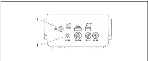
Fig. 36: Transmitter connections
