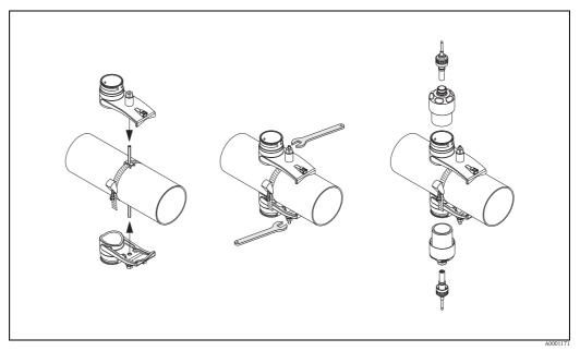
Fig. 31: Steps 1 to 5, installing the sound velocity measuring sensors
