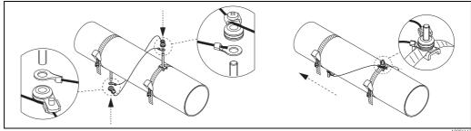
Fig. 23: Positioning the strapping bands (steps 2 to 4)
