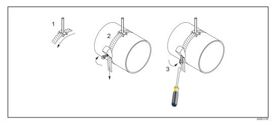
Fig. 16: Premounting strapping bands for pipe diameters  $DN \le 200 (8")$
