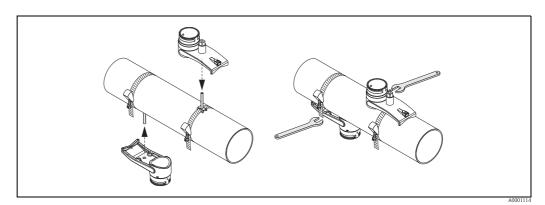
Fig. 24: Mounting the sensor holders
