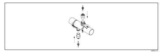
Fig. 26: Mounting the sensor and connecting the connecting cable
