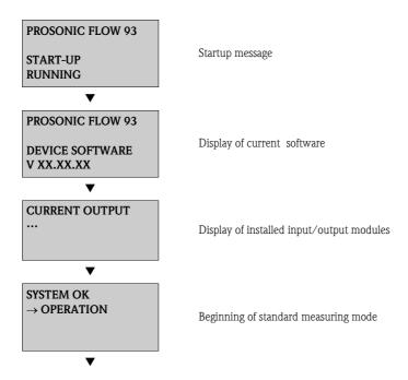
Normal measuring mode commences as soon as startup completes. Various measured value and/or status variables appear on the display (HOME position).
