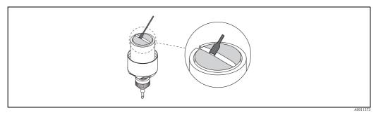
Fig. 29: Coating the contact surfaces of the sensor with coupling fluid
