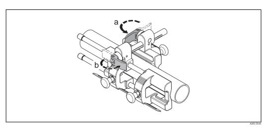
Fig. 15: Fixing the sensor holder
