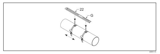
Fig. 27: Determining the distance in accordance with the mounting rail (e.g. POSITION SENSOR G22)
