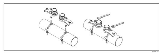
Fig. 28: Mounting the sensor holders
