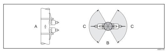
Fig. 4: Recommended orientation and recommended installation range
