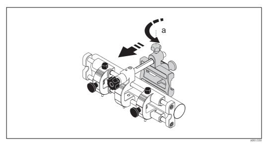
Fig. 10: Guiding the retaining bracket onto the pipe
