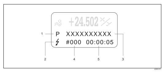
Fig. 40: Error messages on the display (example)
