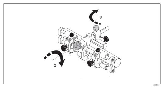
Fig. 11: Fixing the sensor holder
