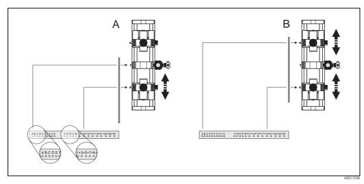
Fig. 8: Setting the sensor distance with the mounting rail (value from POSITION SENSOR function)
