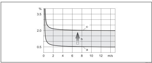
Fig. 44: Example of the measured error in a pipe with a nominal diameter DN > 200 (8")
