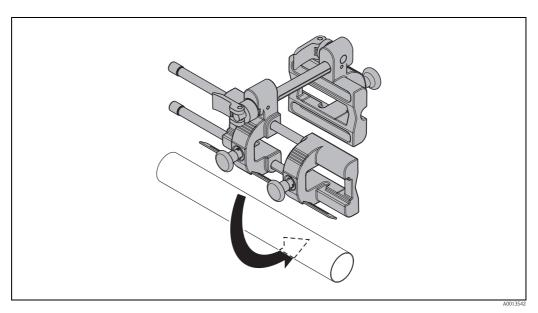
Fig. 13: Setting the sensor holder on the pipe
