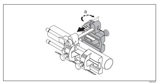
Fig. 14: Guiding the retaining bracket onto the pipe
