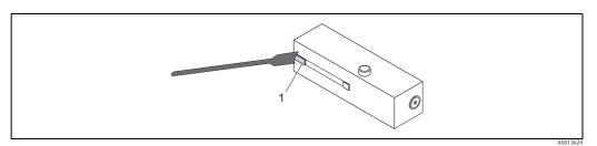
Fig. 19: Coating with coupling fluid
