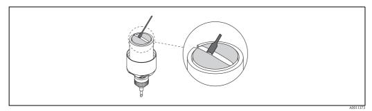
Fig. 25: Coating the contact surfaces of the sensor with coupling fluid
