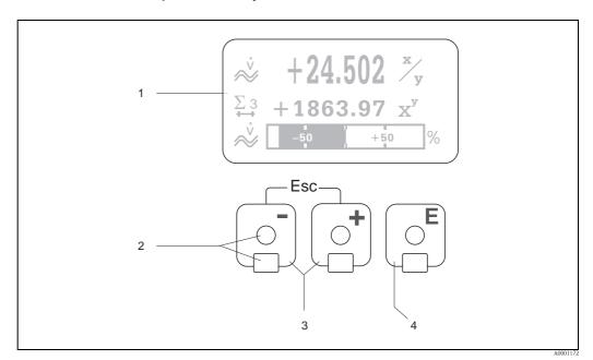
Fig. 37: Display and operating elements
