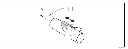
Fig. 35: Measuring the wall thickness
