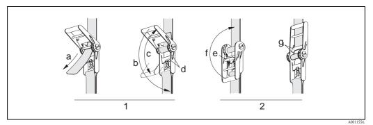
Fig. 18: Strapping band lock
