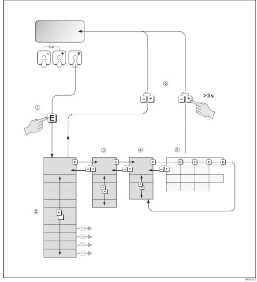
Fig. 39: Selecting functions and configuring parameters (function matrix)
