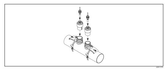
Fig. 30: Mounting the sensor and connecting the connecting cable
