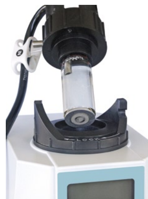
Flow-through cuvette with ultrasonic cleaning
