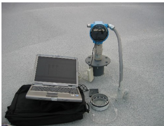
Levelflex M - FMP40 connected to a laptop computer via service adapter to view the current settings and envelope curve
