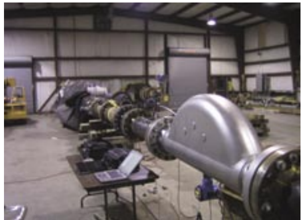
Testing being performed by CEESI of Proline® Promass F 10" Coriolis Mass Flowmeter
