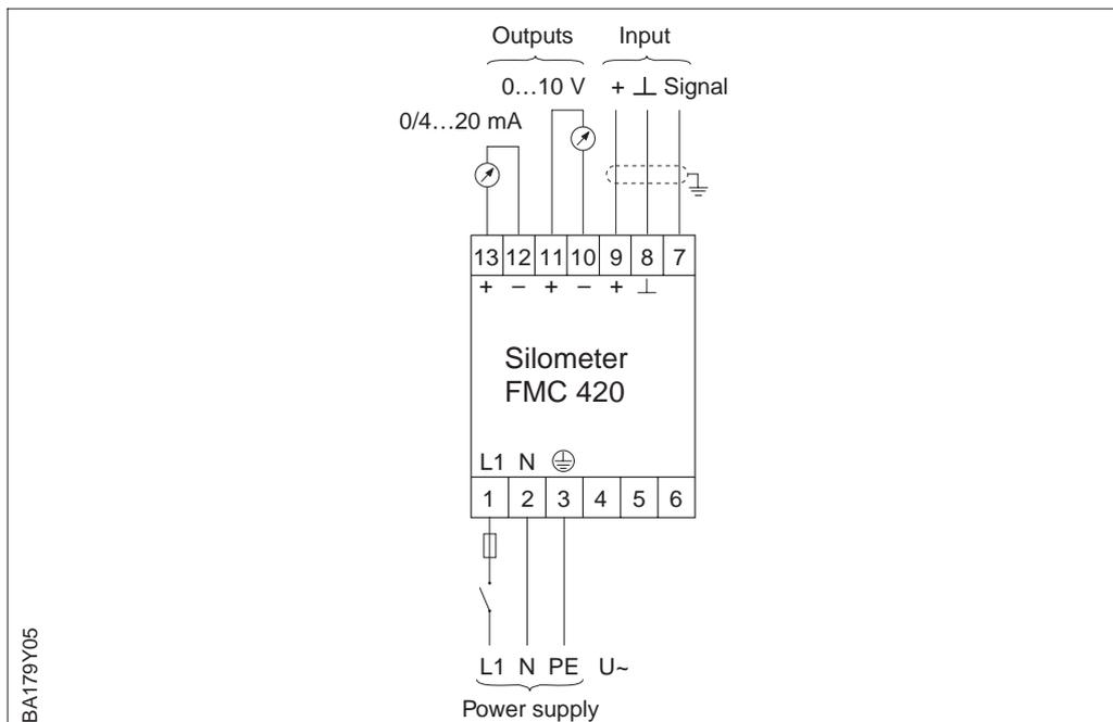
Fig. 5 Electrical connection FMC 420
