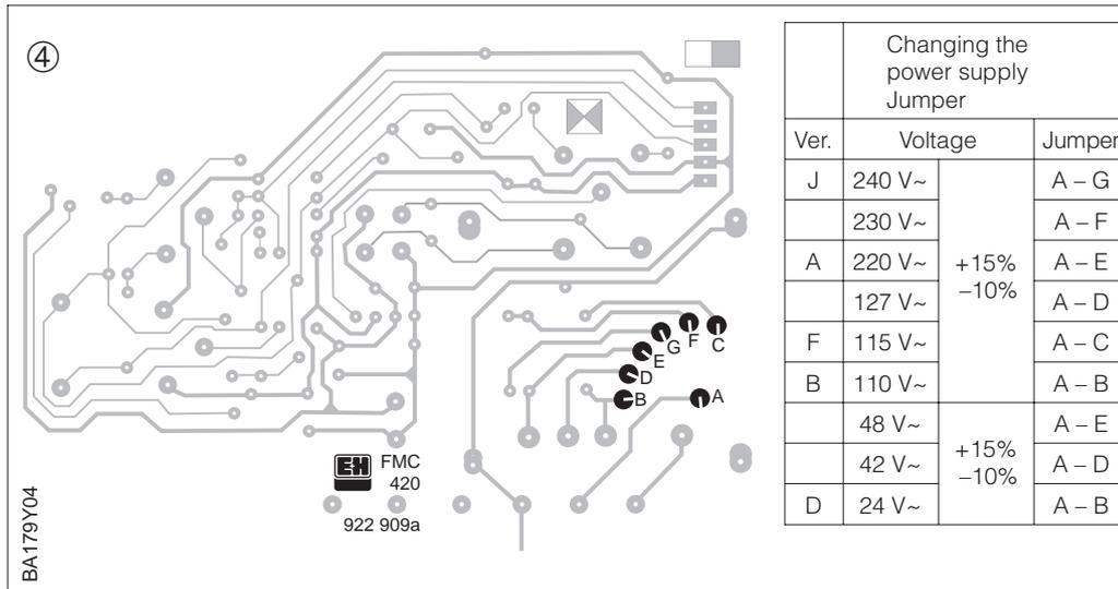
Fig. 4 Changing the power voltage by soldering a jumper onto the circuit board. Versions ("Power supply") see Product Structure on Page 7. Versions J, A, F, B can be set to an AC voltage between 110 V and 240 V, Version D to an AC voltage between 24 V and 48 V.
