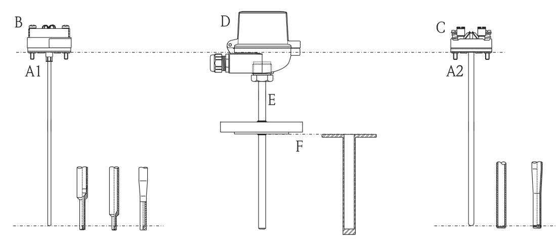
A1 Insert ( $\emptyset$  3 mm, 0.12 in) with mounted head transmitter, for example
