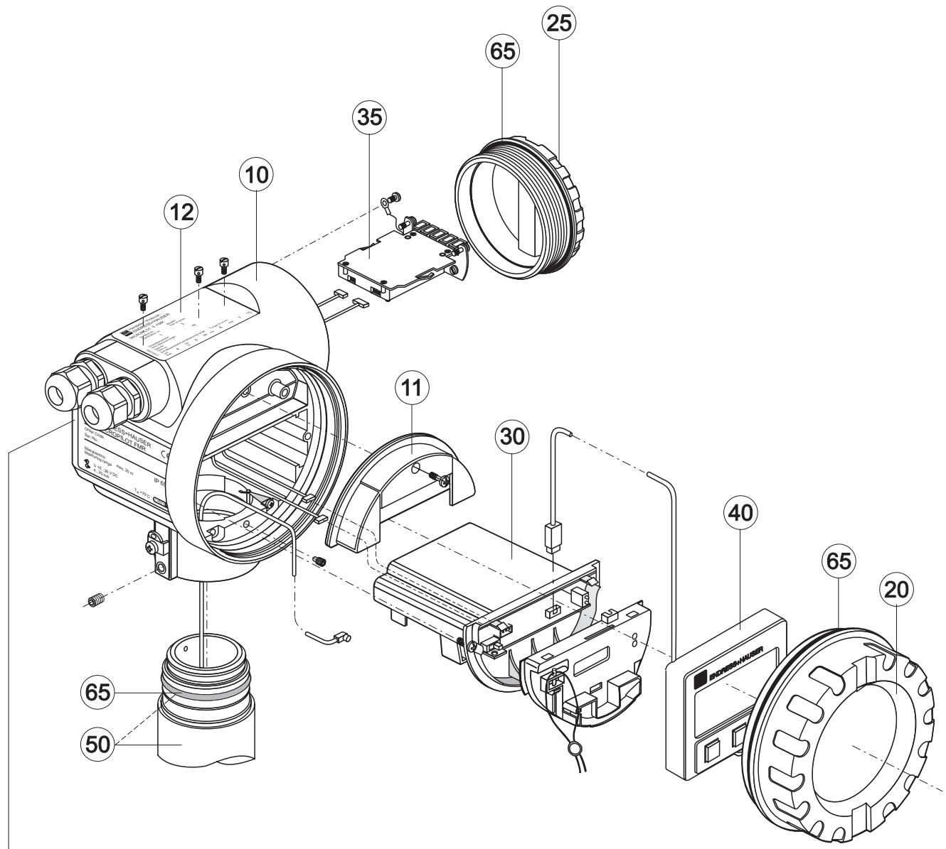
For using in Ex zones cable glands of the generation  $\geq B$  must be required! In addition the permissible temperature range has to be observed ( $> 75^\circ C$ ).
