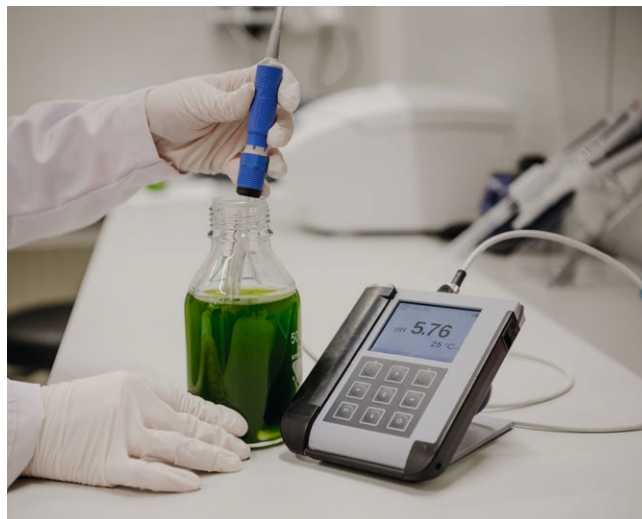
Thanks to the Memosens technology, the same instrumentation can be used in the lab and the production line.
