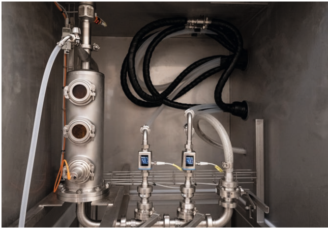
Two Picomag flowmeters with a nominal diameter of DN 20 monitor the volume of beer flowing from the transfer piping to the taps. In the upper left is a Liquicap M FMI51 that continuously monitors the levels.
