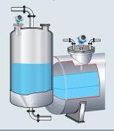
Buffer tank<sup>1)</sup> Agitated surface (e. g. permanent free filling from above, mixing jets)
