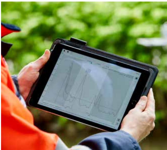
Non-contact commissioning using a tablet and the SmartBlue-app.
