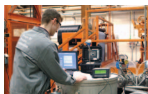
On-site calibration of temperature instruments
