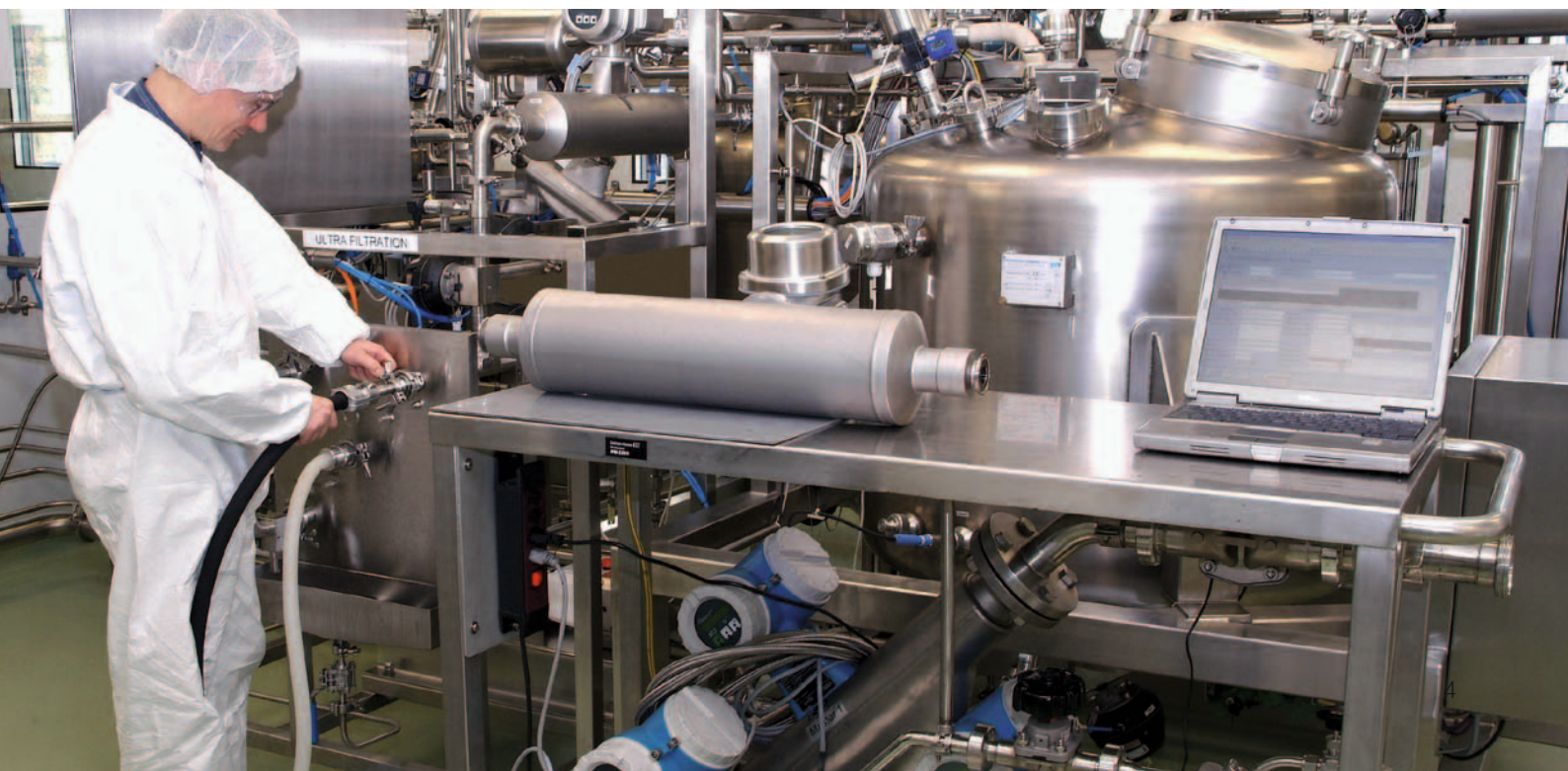
On-site calibration of flowmeters using mobile flow rig
