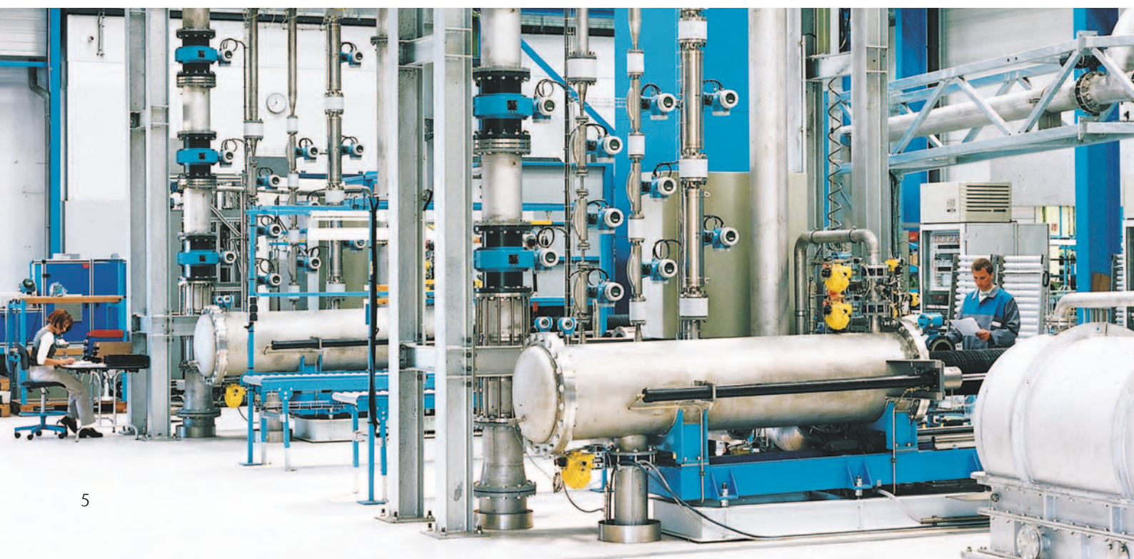
Accredited calibration of flowmeters at Endress+Hauser facilities
