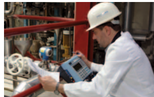
On-site calibration of pressure devices
